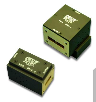
All solid state amplitude and phase matched set consisting of one dual and two single channel receiver protectors. The single channel units are passive. The dual is active with some passive limiting capability. Dual unit includes a driver with BITE for status monitor/ transmitter control.
